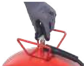
Turn the white valve of the canister counterclockwise until open. Do not close the valve until the canister is empty (this prevents the adhesive curing inside the hose and gun).
