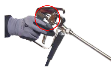
Turn the adjustment screw open and pull the trigger to achieve a consistent spray pattern. Set spray width with the adjustment screw.
